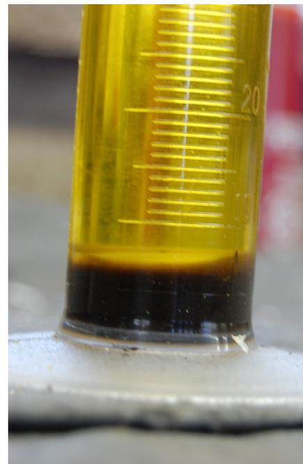
**Fig. 2: 100 milliliters of canola oil collected at pressing time shows about 7 milliliters of sediment after 1 week of settling at room temperature**
