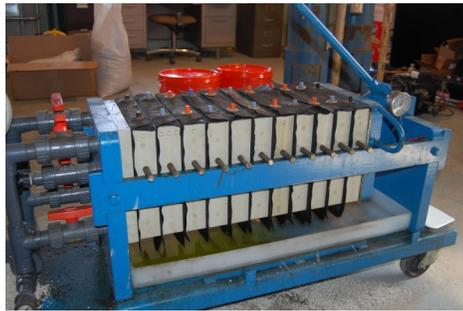
**Fig 7: Filter press; a series of filtering plates are pressed together by manual screw or hydraulic pressure.**
