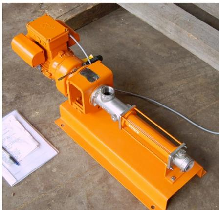
**Fig 10: Electric screw pump for filter press**
