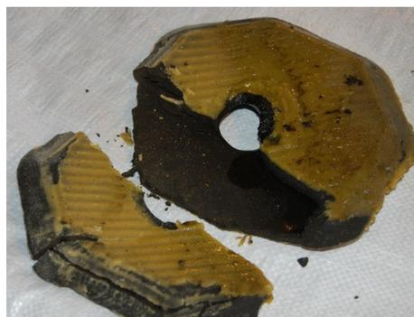
**Fig. 8: Block of foots collected from between two filter press plates. The yellowish colored material is filtering media coating (diatomaceous earth) initially placed on filter plate cloth while the dark colored materials are the foots**
