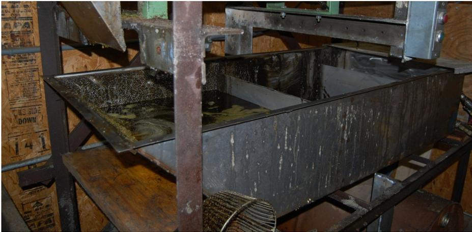
In this tank pressed oil flows slowly from left to right. The oil passes across two partitions, allowing particles time to settle. Most of the settling occurs within the first partition.
