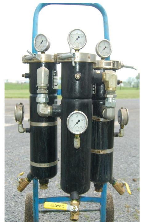
**Fig. 3: Three bag filters and housings arranged in series.**
