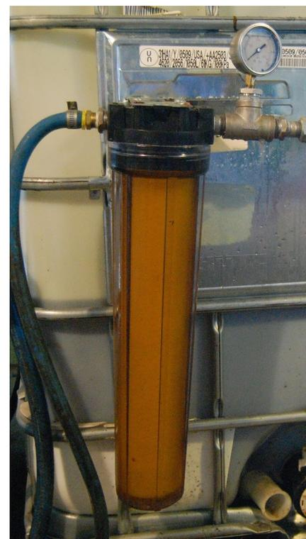
**Fig 6: Cartridge filter with clear housing used as final filter for fueling with straight vegetable oil**
