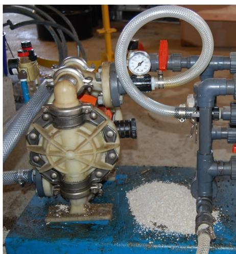
**Fig. 9: Air operated diaphragm pump on filter press**
